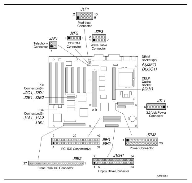
Figure 3. Motherboard Connector Locations
